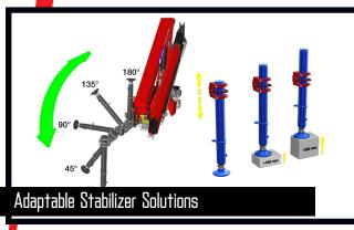
The crane's stabilizer legs are robust, easy to handle and require minimum space. You can choose between fixed stabilizer legs or manual swing-up stabilizer legs (45°, 90°, 135°, 180°) with or without gas spring. The stabilizer cylinder is adjustable by +/- 200 mm in height, with full stroke.
